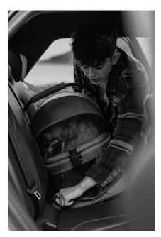
Pull the seat belt through the loops on the longest side and plug the seat belt into the buckle to secure in place.
